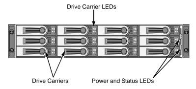
Figure 2. VTrak M300f/i/p front view (M200f/i/p is similar)
